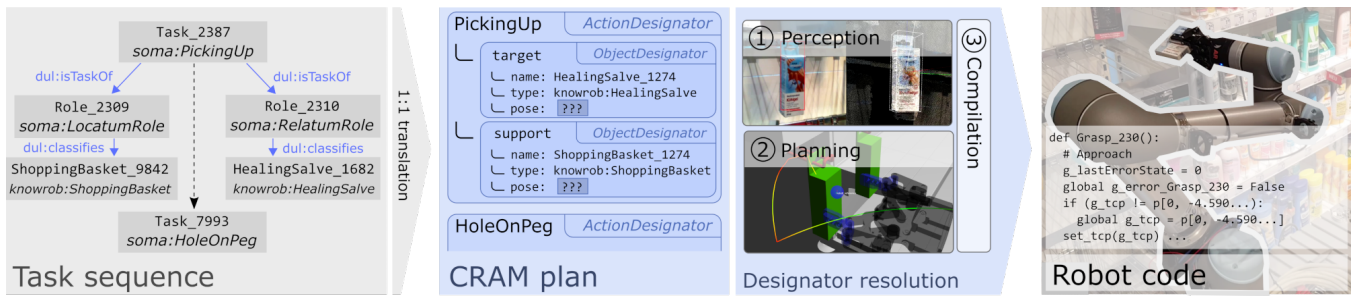
Figure 5: The proposed program generation pipeline. A sequence of Tasks is translated into an underspecified plan (here, the real-world poses of the healing salve and shopping basket are not known a priori). Via reasoning, perception and collision-free motion planning, the plan is ultimately resolved to native robot code.
